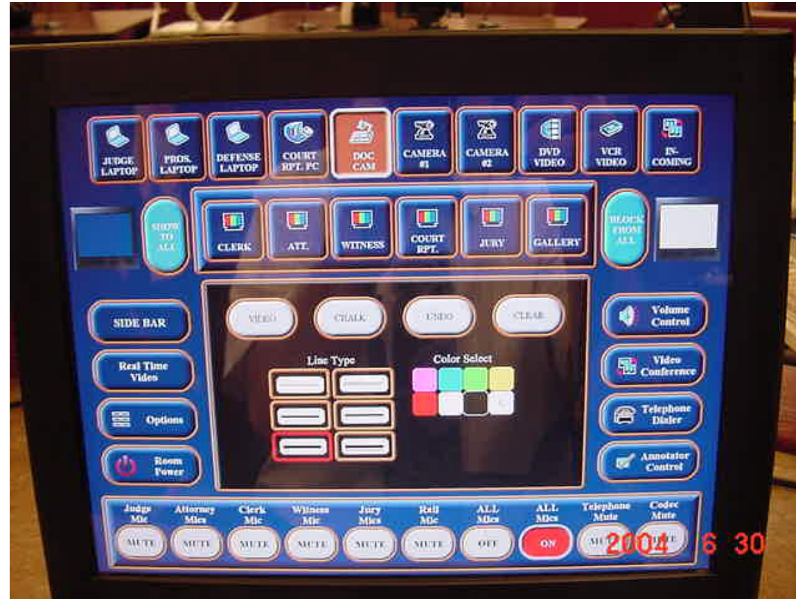
Fig. 4: The control panel for the e-courtroom, which sits on the bench. In addition to controlling the monitors and microphones in the courtroom, the Court also activates ITV through this panel.
