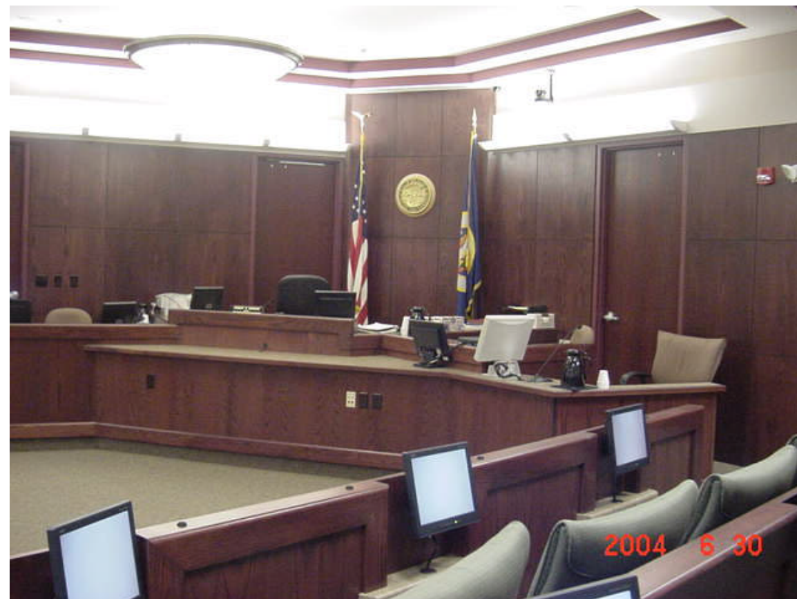
Fig.27-Monitors in front of the jurors. The jurors can not only see video and objects projected through the document camera, but also any other video source, including Interactive Television
