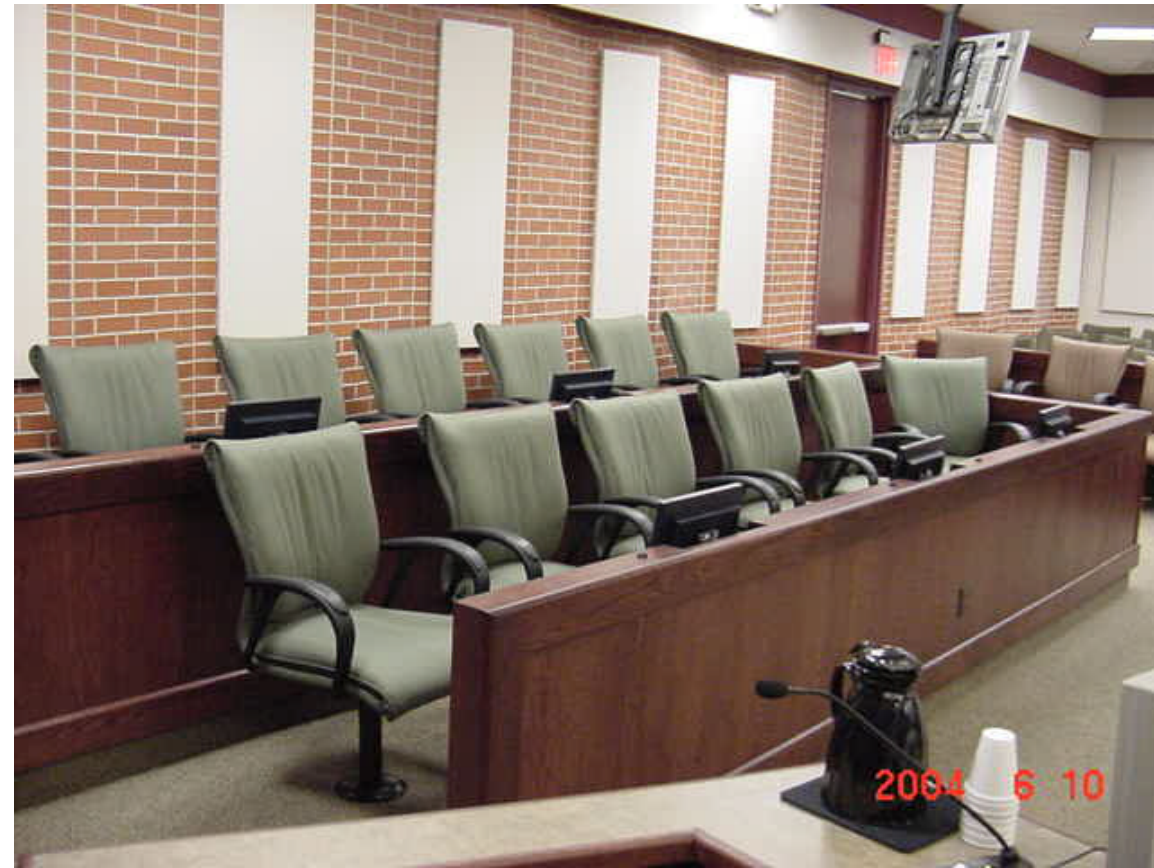
Fig. 12: Jury box, showing the shared monitors. Note that the monitors are low and slightly tilted up.
